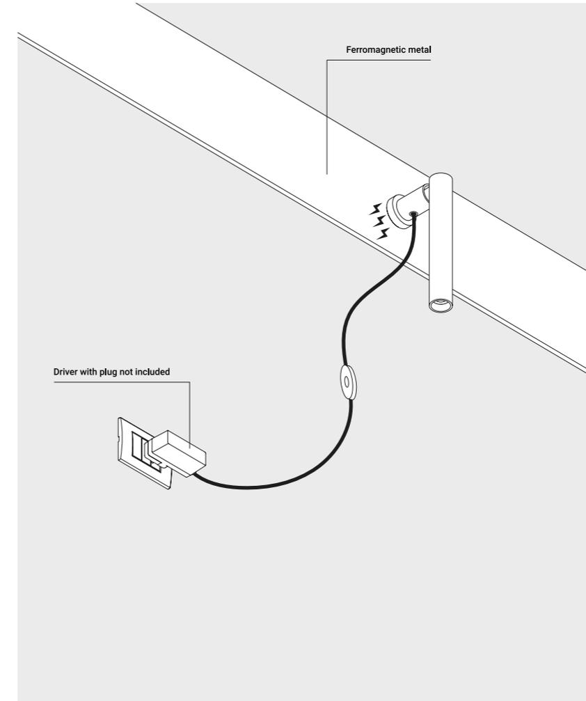
1A3180300.00.06 - 1A3180400.00.06 - Example of installation with driver with plug
